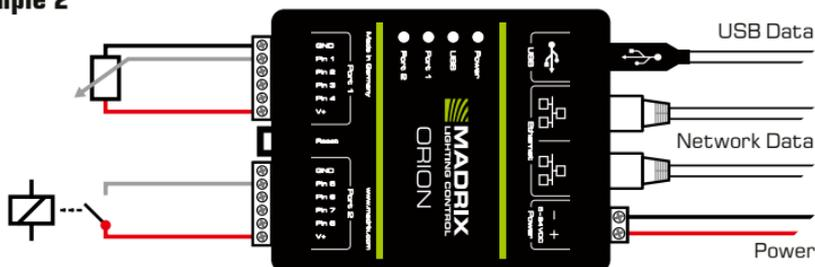
**Description:** This diagram is based on Example A and adds a relay as switch to Port 2. This relay creates a potential-free separation (galvanic isolation) and allows using different voltages or AC, for example. This only works if power is supplied externally to the device via Power. Please see above for more information.
